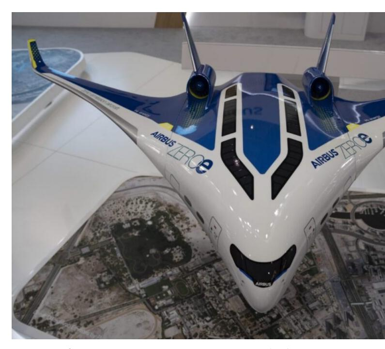
The Airbus ZEROe principles are all hybrid-hydrogen airplane and consistof the following setups: turbofan, turboprop, and blended-wing body (pictured above). (Airbus)
